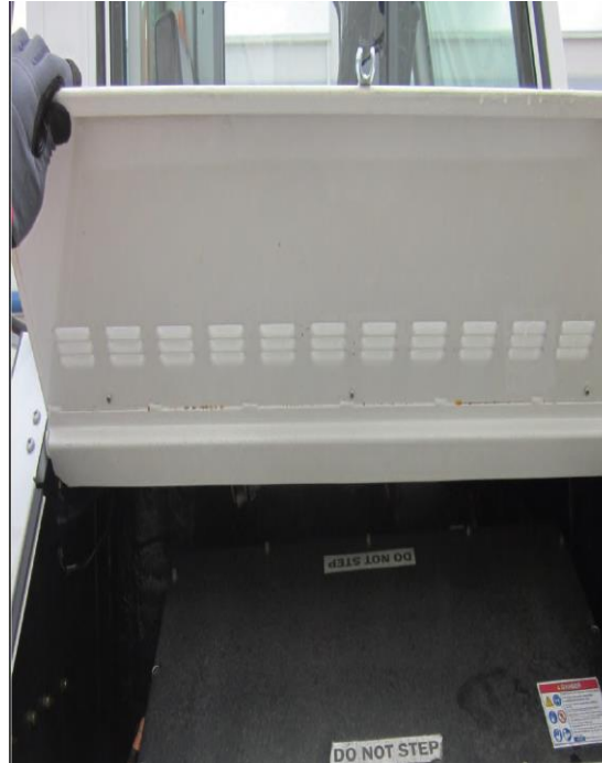
Terminal Tractor Electrical Component Compartment
