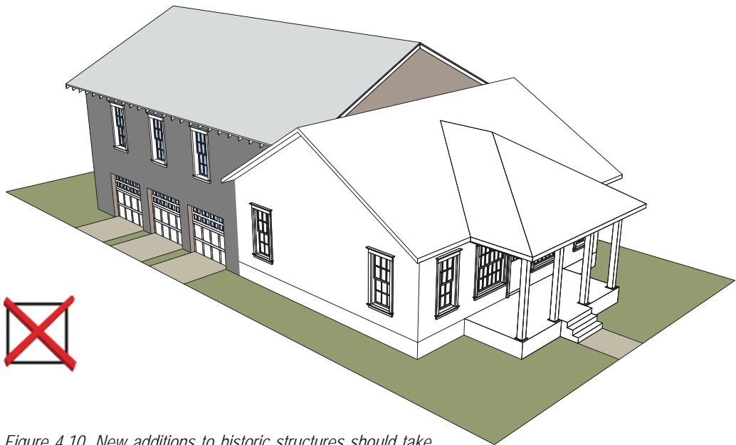
Figure 4.10. New additions to historic structures should take care to retain the integrity of the original structure, there should be a clear distinction between the addition and the original.
