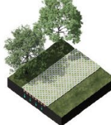
Permeable Pavers / Surfaces
