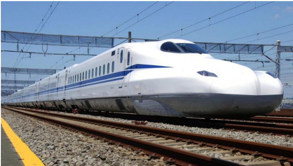
Figure 13: JR Shinkansen N700 with Overhead Contact System
