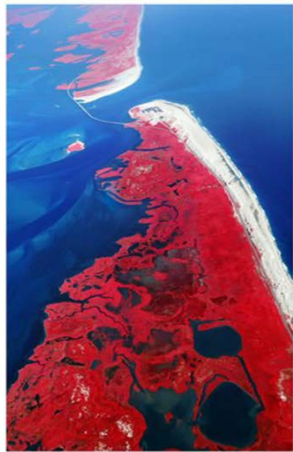
Figure 7. A comparison of panchromatic (left image), color (middle image), and CIR (right image) of North Carolina's Oregon Inlet from the north end of Pea Island looking north. CIR imagery depicts clear, blue water as black, since water absorbs NIR wavelength energy. Water with varying amounts of suspended particles appears in CIR imagery as shades of blue, because suspended particles reflect a very small amount more of green light than clear water does. Photo source: NCDOT Photogrammetry Unit. The three images were acquired in one pass on 10 August 2010 with an Intergraph Digital Mapping Camera.
