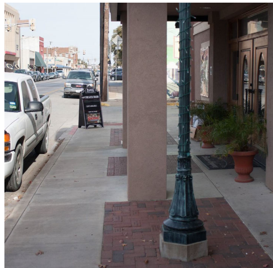
Brick pavers, planters, and decorative lighting influence the aesthetic character of this sidewalk, but can also present obstacles for pedestrians. Location: Plaza Theater on Mill Street
