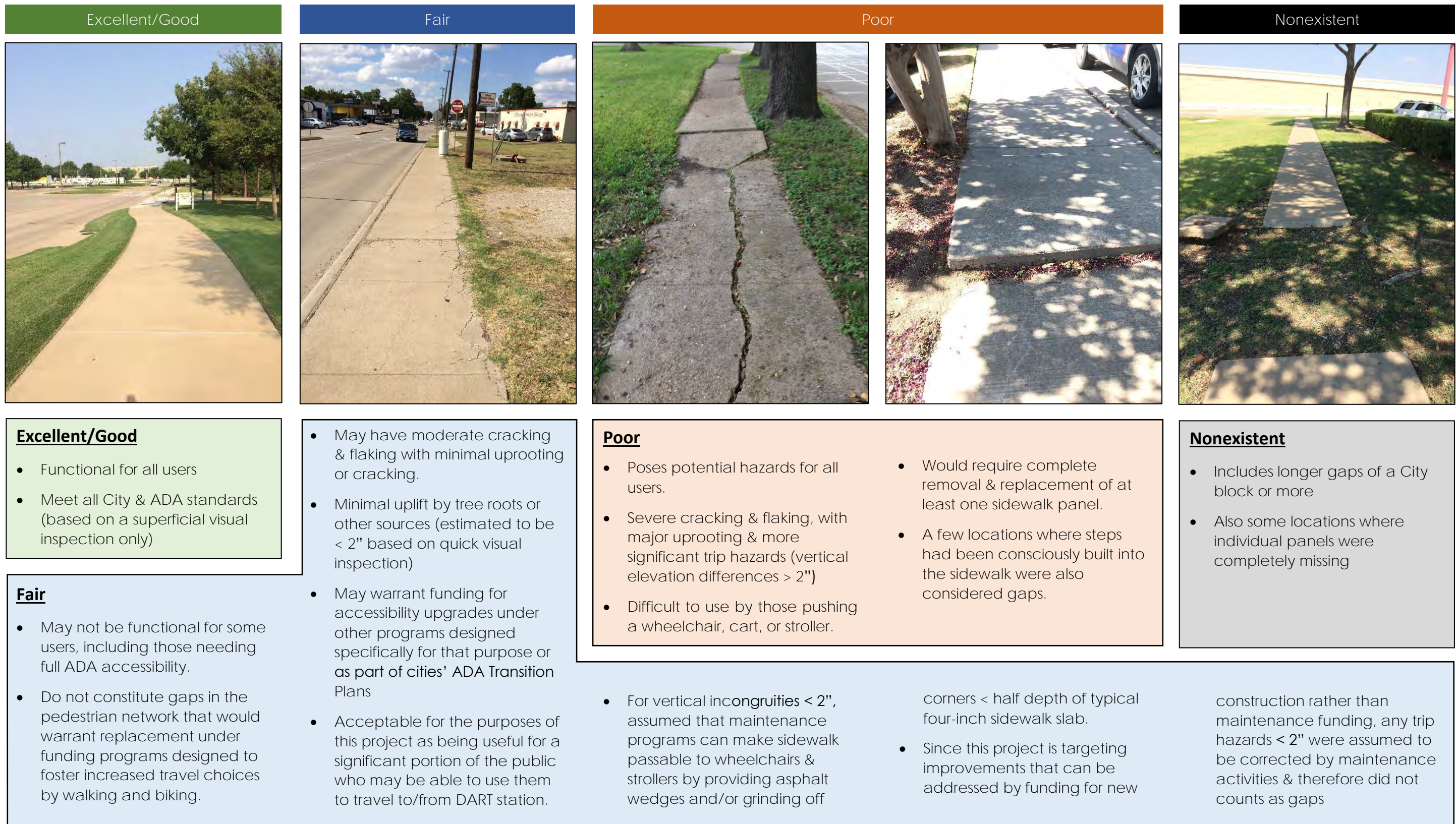
Figure 3: Sidewalk Condition Classification
