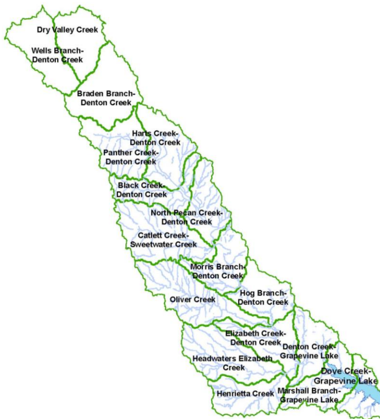
Figure A.9: The 17 subwatersheds (defined by the green polygons) that make up the Grapevine Lake watershed. Stream segments are only mapped for those areas within the 16-county North Central Texas region.
