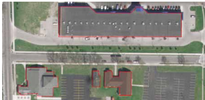
Figure 5. 3D roof boundaries are clearly identified
