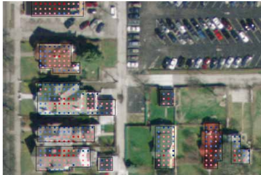
Figure 9. Solar energy potential map (red points represent the highest potential; pink, medium; and blue, lowest)
