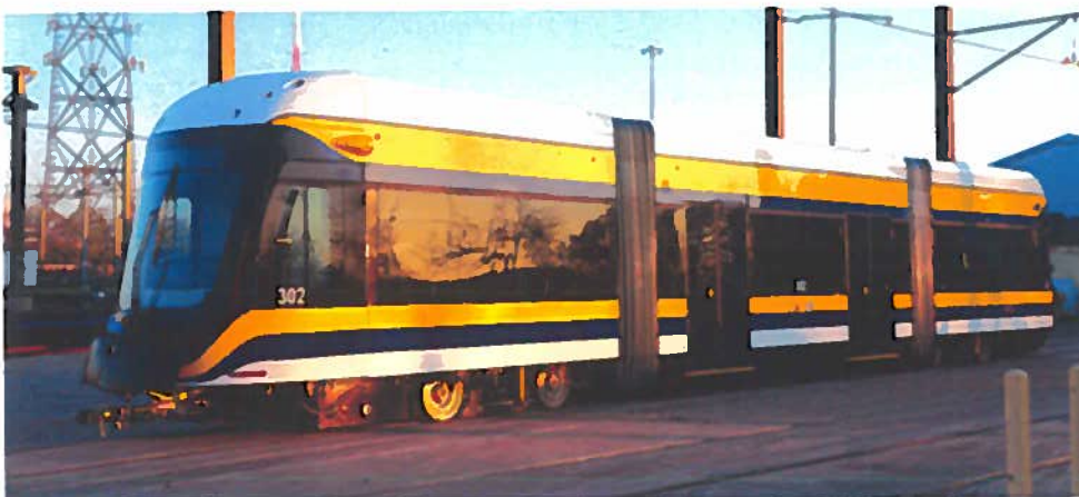
The Dallas Streetcar vehicles, designed and built by Brookville Equipment Corp. of Pennsylvania, will be the first dual-mode streetcars built in the U.S.
