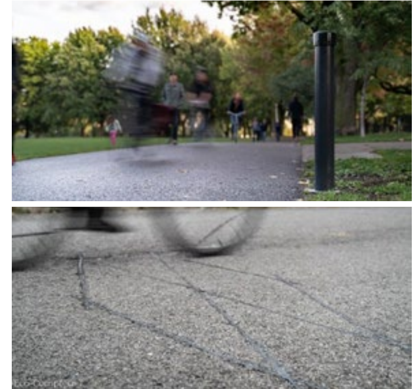
Examples of dual activity counters. The top image shows the infrared sensor, and the bottom image shows the wire, or inductive loop cyclist detector. Both images from Eco-Counter
