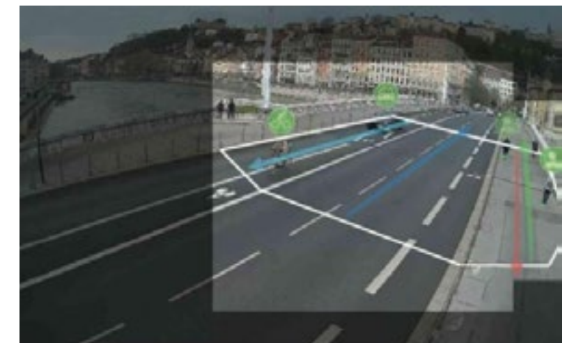
Example of a video detection counter. The top image shows the installed detector, and the bottom image shows what the camera is detecting. Both images from Eco-Counter
